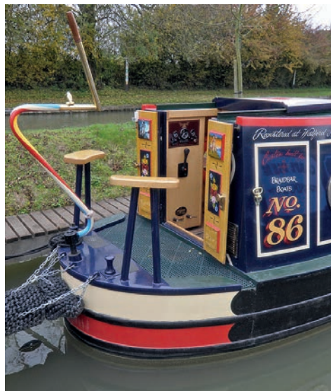
Differing styles of stern: Semi trad style (left) and Trad style (above). Photos courtesy of ABNB
